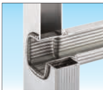
30 x 30 mm square-section non-slip rungs with double edging
