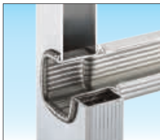
30 x 30 mm square-section non-slip rungs with double edging Rung connection to the upright with double edging, on the inside and outside, for maximum protection against accidental impact and long-lasting use
