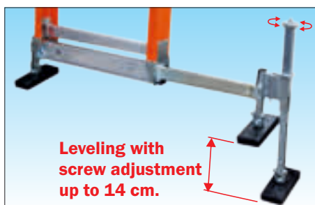
Base equipped with 1 leveling foot in galvanized steel with screw adjustment and tilting foot that can be assembled and disassembled if necessary to bridge slopes or unevenness with ease and precision
