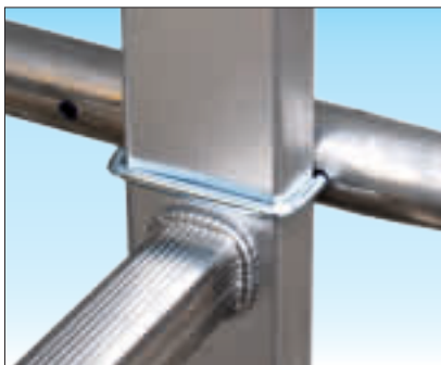
Adjustable fixing of cage hoops by means of stainless steel U-bolts and self-lubricating nylon washers
