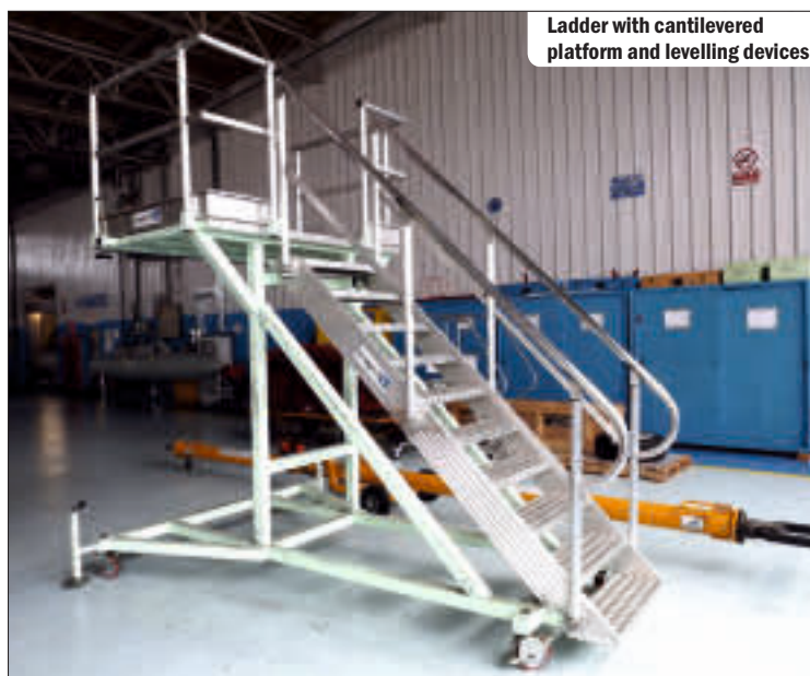
Special stepladder with self-deactivating wheels
