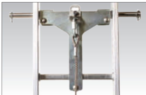
Upper fixing plate with anchor point equipped with snap hook and Ø 25 mm tube, for step reinforcement
