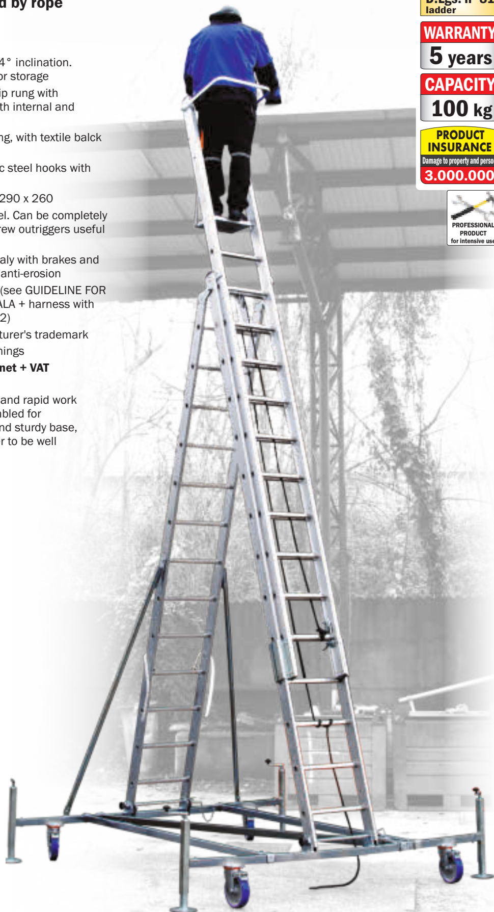
30 x 30 mm square-section non-slip rungs with double edging Rung connection to the upright with double edging, on the inside and outside, for maximum protection against accidental impact and long-lasting use
