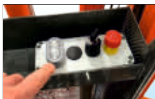
Control panel and push-button panel on the basket
